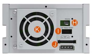
A. Mute Button B. HDD status indicator LED C. Key Lock D. HDD tray E. LCD Display F. RAID Setting Button G. Alarm indicator LED H. RS232 Port I. 3.5" HDD SATA Port (for host) J. Power Socket K. Cooling Fan
